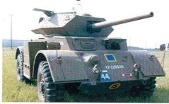
This 1942 Staghound version T17E1 was designed for armoured and reconnaissance regiments for both short and long distance operations. It was also used for special missions such as raids, securing tactical positions and the protection of headquarters and convoys. Variations of armament included the basic 37mm gun, 3 inch howitzer, 75mm tank gun and the twin .50 calibre machine gun for the anti-aircraft role. This vehicle was manufactured by General Motors.
