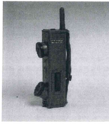
Galvin Manufacturing Corporation (later Motorola) Handie-Talkie SCR536 portable two-way radio, circa 1940.
