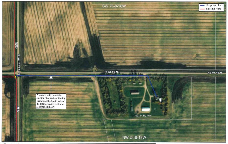
Offset of Fibre distribution and Handhole Vaults are 3m (unless otherwise specified) from adjacent property line within ROW Hand hole Vaults are 2 ft by 3ft and are flush with ground level.
