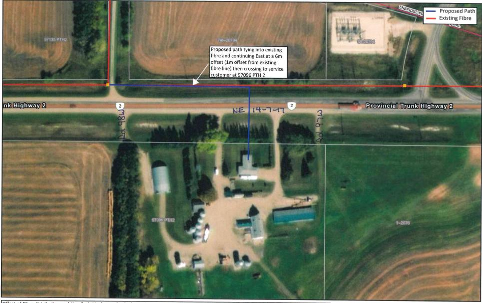
Offset of Fibre distribution and Handhole Vaults are 6m (unless otherwise specified) from adjacent property line within ROW Hand hole Vaults are 2 ft by 3ft and are flush with ground level.
