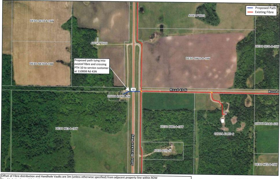
Hand hole Vaults are 2 ft by 3ft and are flush with ground level.
