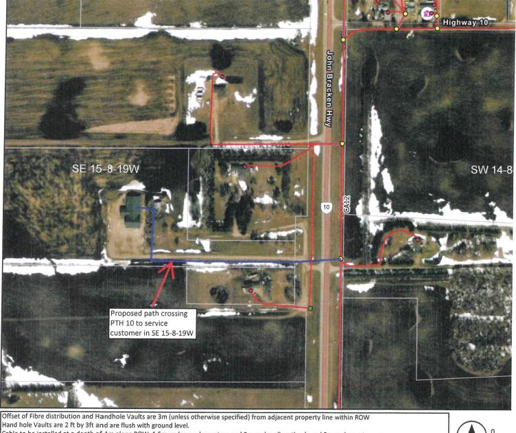
Cable to be installed at a depth of 1m along ROW, 1.5m under road crossings and 2m under all wetlands and 3m under water runs. Where the fibre optic cable crosses provincial roads, municipal roads, turning lanes, private access lanes, field crossings, wetland areas and water runs, RFNOW Inc. shall install the cable by means of directional bore;
