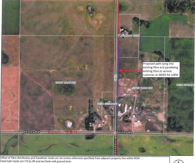
Hand hole Vaults are 2 ft by 3ft and are flush with ground level. Cable to be installed at a depth of 1m along ROW, 1.5m under road crossings and 2m under all wetlands and 3m under water runs.
